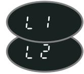
**L2** Lock Mode (disables the jets and light buttons to prevent unauthorized use of the hot tub) - filter cycles and heater will continue to operate as programmed in this mode. The temperature display flashes when this function is enabled. Example: the “F3” filter cycle was enabled prior to choosing lock mode. The hot tub continues to perform filter cycle “F3” until lock mode is canceled, allowing another filter cycle to be selected.
