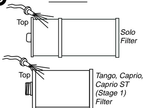
Rinse debris from all filter pleats using a garden hose and high-pressure nozzle. Start at top and work downward to face. Repeat process until all filter pleats are clean.
