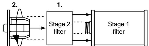
1. Install stage 2 filter onto clean stage 1 filter.
