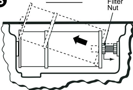
Loosen filter nut to provide clearance, then remove filter assembly.
