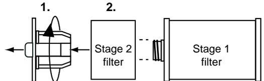
1. Rotate stage 2 retainer **counterclockwise** to release, then separate filter assembly.
