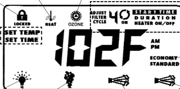
Indicates hot tub light is on (changes according to brightness selected).
